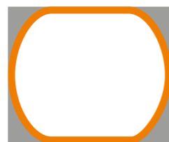
Flat Oval Tube (weight reduction: > 21%)
